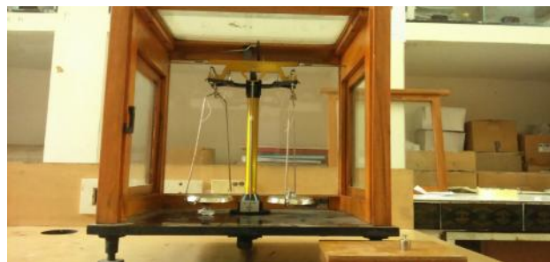
Fig 1 : Measurement of bioadhesive strength by physical balance
