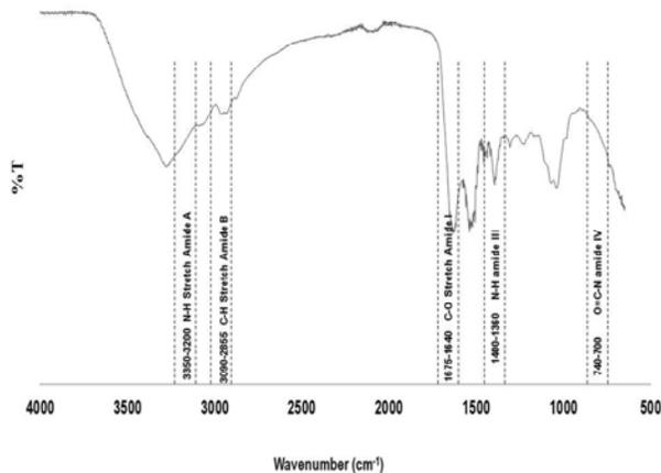
Fig 7: The FTIR Spectra of Freeze Dried AMSC-MP
