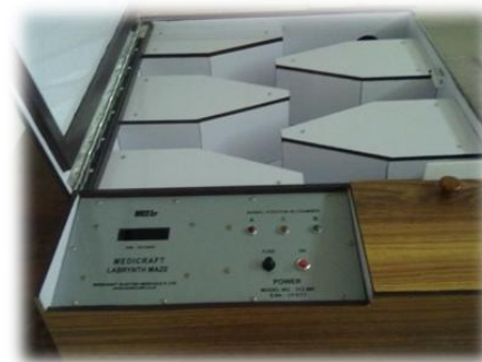
Fig 3&4: Digital count screen and electrical indicator for showing animal presence
