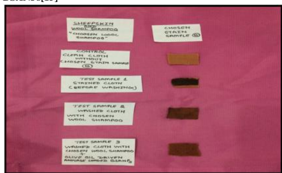
Fig 3: Washing results of stained woolen fabric pieces having chosen stain sample B of hair color dye crème (Garnier Nutrisse Nourishing Color Crème Black) with chosen wool shampoo named, Wool Shampoo for Sheepskin and Wool Products and prepared bio-active olive oil driven amylase loaded BSANPs 15
